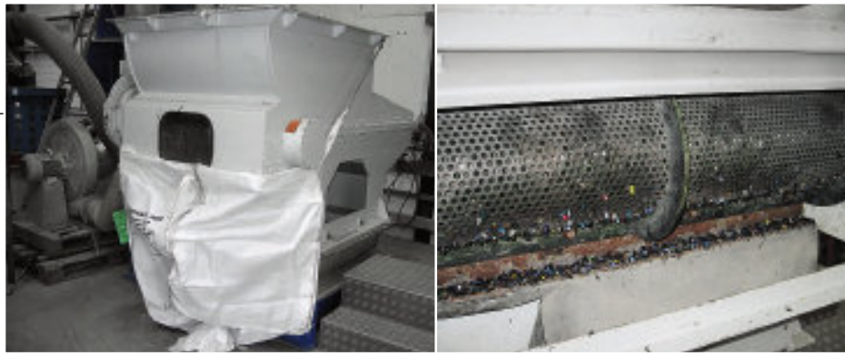
Fig. 1 Shredder for the reduction of the capacitors (type: Vecoplan VAZ 105/120, 18.5 kW, approx. 550 kg/h) and 8 mm sieve used for IT/CE < 1 cm (bulk sample N° 7)
