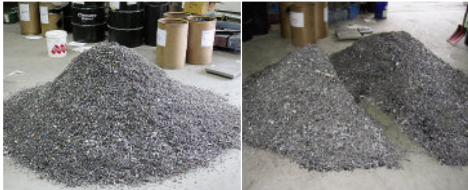
Fig. 2 Splitting and reduction of samples by means of splitting the angle of repose of the shredded material
